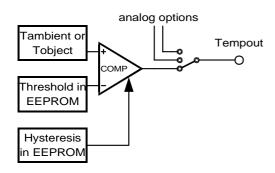
The comparator is a digital comparator, with a resolution of 12 bits. By default the input polarity is inverting. The default threshold and hysteresis values are version dependent, as indicated below.
