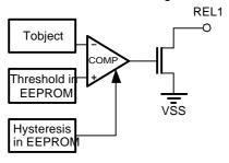
The comparator is a digital comparator, with a resolution of 12 bits. By default the input polarity is inverting. By default the trigger temperature is the object temperature but also the ambient (sensor) temperature can be used. Threshold and hysteresis values are version dependent, as indicated below.
